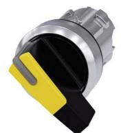
Selector switch, illuminable, 22 mm, round, metal, shiny, yellow, selector switch, long, 2 switch positions O<I, momentary contact type, Actuating angle 45°, 10:30h/12h, Z=50-unit packaging
