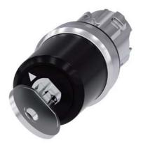
key-operated switch Siemens, 22 mm, round, metal, shiny, lock number SSG10, with 2 keys, 2 switch positions O-I, latching, actuating angle 90°, 10:30h/13:30h, key removal I, Z=50-unit packaging
