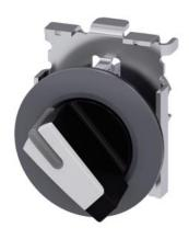
Selector switch, illuminable, 30 mm, round, Metal, matte, white, selector switch, short, front ring for flush installation, 2 switch positions O<I, momentary contact type, Actuating angle 45°, 10:30h/12h, with laser labeling, lower case
