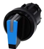
Selector switch, illuminable, 22 mm, round, plastic, blue, selector switch, short, 3 switch positions I>O<II, momentary contact on the left, latching on the right, actuating angle  $2x45^{\circ}$ , 10:30h/12h/13:30h, with laser labeling, lower case
