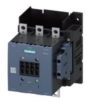
Power contactor, AC-3 150 A, 75 kW / 400 V without coil Auxiliary contacts 2 NO + 2 NC 3-pole, Size S6 Busbar connections Drive: conventional Auxiliary conductor: Screw terminals
