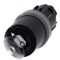
Key-operated switch IKON, 22 mm, round, plastic with metal front ring, lock number 360012K1, with 2 keys, 2 switch positions O-I, latching, actuating angle 90°, 10:30h/13:30h, key removal O, Z=50-unit packaging
