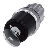
Key-operated switch BKS, 22 mm, round, metal, shiny, Lock No. E9 (VW), without key, 2 switch positions O-I, latching, actuating angle 90°, 10:30h/13:30h, key removal O+I, Z=50-unit packaging
