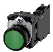
Pushbutton, 22 mm, round, plastic, green, pushbutton, flat, momentary contact type, with holder 1 NO+1 NC, spring-type terminal, with laser labeling, upper case and lower case, always upper case at beginning of line
