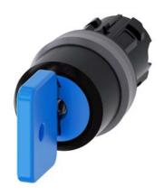
Key-operated switch O.M.R, 22 mm, round, plastic with metal front ring, lock number 73038, blue, with 2 keys, 3 switch positions I-O<II, left latching, right momentary contact type, actuating angle 2x45°, 10:30h/12h/13:30h, key removal O, with laser labeling, upper case and lower case, always upper case at the beginning of the word
