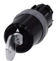
key-operated switch Siemens, 22 mm, round, plastic with metal front ring, lock number SSG10, with 2 keys, 3 switch positions I-O<II, left latching, momentary contact type on the right, actuating angle 2x45°, 10:30h/12h/13:30h, key removal I, with laser labeling, upper case and lower case, always upper case at beginning of line
