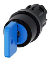
Key-operated switch O.M.R, 22 mm, round, plastic, lock number 73038, blue, with 2 keys, 3 switch positions I-O<II, left latching, right momentary contact type, actuating angle 2x45°, 10:30h/12h/13:30h, key removal O, with laser labeling, Customer-specific selection with SIRIUS ACT configurator (CIN)
