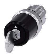
Key-operated switch BKS, 22 mm, round, metal, shiny, lock number S1, with 2 keys, 3 switch positions I>O<II, momentary contact on the left, latching on the right, actuating angle  $2x45^{\circ}$ , 10:30h/12h/13:30h, key removal O, Z=50-unit packaging
