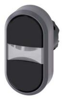
Twin pushbutton, 22 mm, round, plastic with metal front ring, black, black, pushbuttons, flat, with laser labeling, inscription or symbol Customer-specific selection with SIRIUS ACT configurator (CIN)
