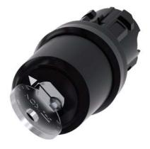
Key-operated switch IKON, 22 mm, round, plastic, special lock, with 2 keys, 2 switch positions O<I, momentary contact type, Actuating angle  $45^\circ,\,$  10:30h/12h, Key removal O
