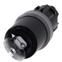
Key-operated switch IKON, 22 mm, round, plastic with metal front ring, lock number 360012K1, with 2 keys, 2 switch positions O<I, momentary contact type, Actuating angle 45°, 10:30h/12h, key removal O, with laser labeling, upper case and lower case, always upper case at beginning of line
