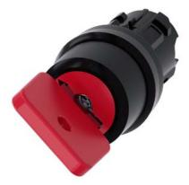
Key-operated switch O.M.R, 22 mm, round, plastic, lock number 73037, red, with 2 keys, 2 switch positions O<I, momentary contact type, Actuating angle 45°, 10:30h/12h, key removal O, with laser labeling, upper case
