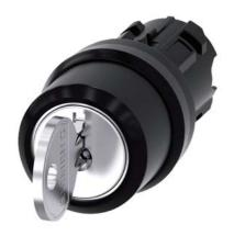
RONIS key-operated switch, 22 mm, round, plastic, special lock, with 2 keys, 3 switch positions I-O<II, left latching, right momentary contact type, actuating angle  $2x45^{\circ}$ , 10:30h/12h/13:30h, key removal O+I, possible special locks: SB31, 421, 455
