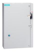
Non-reversing motor starter, Size 2 1/2, Three phase full voltage, Solidstate overload relay, OLR amp range 25-100A, Combination type, 100A fusible disconnect, 100A/250V fuse clip, Enclosure NEMA type 1, Indoor general purpose use, Extra-wide enclosure
