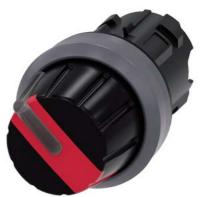
Selector switch, illuminable, 22 mm, round, plastic with metal front ring, red, Rotary knob, 2 switch positions O-I, latching, actuating angle 90°, 10:30h/13:30h, with laser labeling, lower case
