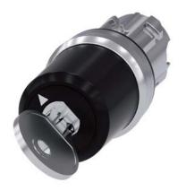
Key-operated switch BKS, 22 mm, round, metal, shiny, lock number S1, with 2 keys, 2 switch positions O-I, latching, actuating angle 90°, 10:30h/13:30h, key removal O+I, with laser labeling, inscription or symbol Customer-specific selection with SIRIUS ACT configurator (CIN)
