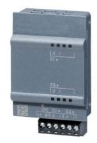
SIPLUS S7-1200 SB 1223 2DI/2DQ based on 6ES7223-0BD30-0XB0 with conformal coating, -40...+60 °C, start up -25 °C, digital input/output 2 DI 24 V DC/2 DQ 24 V DC
