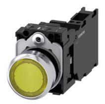
Illuminated pushbutton, 22 mm, round, metal, shiny, yellow, pushbutton, flat, momentary contact type, with holder, 1 NO+1 NC, LED module with integrated LED 230 V AC, spring-type terminal, Z=20-unit packaging
