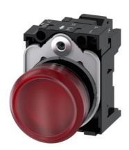
Indicator lights, 22 mm, round, plastic, red, lens, smooth, with holder, LED module, with integrated LED 230 V AC, spring-type terminal, with laser labeling, lower case
