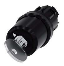
key-operated switch Siemens, 22 mm, round, plastic, lock no. LSG1, with 2 keys, 2 switch positions O-I, latching, actuating angle  $90^\circ$ , 10:30h/13:30h, key removal O, with laser labeling, upper case and lower case, always upper case at beginning of line
