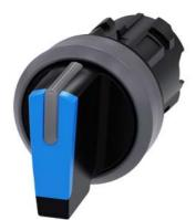
Selector switch, illuminable, 22 mm, round, plastic with metal front ring, blue, selector switch, short, 3 switch positions I-O<II, left latching, right momentary contact type, actuating angle 2x45°, 10:30h/12h/13:30h, with laser labeling, inscription or symbol Customer-specific selection with SIRIUS ACT configurator (CIN)
