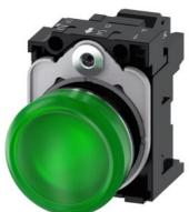
Indicator lights, 22 mm, round, metal, shiny, green, lens, smooth, with holder, LED module with integrated LED 110 V AC, spring-type terminal, with laser labeling, upper case
