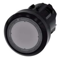
Indicator light in illuminated pushbutton design, 22 mm, round, plastic, clear, with laser labeling, upper case and lower case, always upper case at beginning of line
