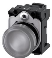
Indicator lights, 22 mm, round, Metal, shiny, clear, lens, smooth, with holder, LED module with integrated LED 230 V AC, spring-type terminal, with laser labeling, symbol number according to, ISO 7000 or IEC 60417
