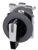
Selector switch, illuminable, 30 mm, round, Metal, matte, white, selector switch, long, front ring for flush installation, 3 switch positions I-O-II, latching, actuating angle 2x45°, 10:30h/12h/13:30h, with laser labeling, upper case
