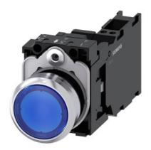
Illuminated pushbutton, 22 mm, round, metal, shiny, blue, pushbutton, flat, momentary contact type, with holder, 1 NO+1 NC, LED module with integrated LED 24 V AC/DC, spring-type terminal, with laser labeling, upper case and lower case, Always upper case at the beginning of the word
