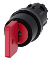
Key-operated switch O.M.R, 22 mm, round, plastic, lock number 73037, red, with 2 keys, 3 switch positions I>O<II, momentary contact type, actuating angle 2x45°, 10:30h/12h/13:30h, Key removal O Z=50-unit packaging
