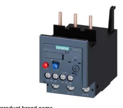
Overload relay 22...32 A Thermal For motor protection Size S2, Class 10 Contactor mounting Main circuit: Screw Auxiliary circuit: Screw Manual-Automatic-Reset
