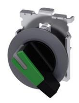
Selector switch, illuminable, 30 mm, round, Metal, matte, green, selector switch, long, front ring for flush installation, 2 switch positions O-I, latching, actuating angle  $90^\circ$ , 10:30h/13:30h, with laser labeling, upper case
