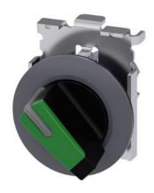
Selector switch, illuminable, 30 mm, round, Metal, matte, green, selector switch, short, front ring for flush installation, 2 switch positions O-I, latching, actuating angle  $90^\circ$ , 10:30h/13:30h, with laser labeling, upper case
