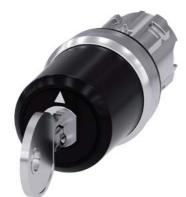
key-operated switch Siemens, 22 mm, round, metal, shiny, special lock, with 2 keys, 3 switch positions I>O<II, momentary contact on the left, latching on the right, actuating angle  $2x45^{\circ}$ , 10:30h/12h/13:30h, key removal II
