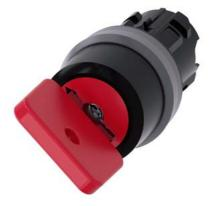
Key-operated switch O.M.R, 22 mm, round, plastic with metal front ring, lock number 73037, red, with 2 keys, 2 switch positions O-I, latching, actuating angle  $90^\circ,\,10:30h/13:30h,$  key removal O, with laser labeling, upper case and lower case, always upper case at the beginning of the word
