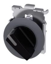
Illuminable selector switch, 30 mm, round, Metal matte, black, Selector switch short, front ring for flush installation, momentary contact type, Actuating angle  $45^\circ,\,10:\!30h/12h$
