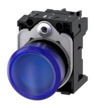
Indicator light, 22 mm, round, plastic, blue, lens, smooth, with holder, LED module, with integrated LED 24 V AC/DC, screw terminal, with laser labeling, upper case and lower case, always upper case at beginning of line
