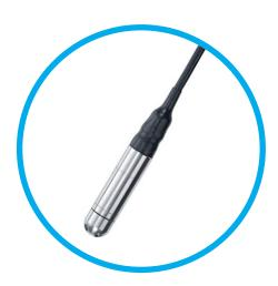
The ILTS is designed for use in continuous submersion in liquids such as water, oil and fuels. The probe uses the latest piezo-resistive media-isolated silicon sensing technology and a stainless steel diaphragm. Housed within a 316L stainless steel, or high grade Duplex stainless steel housing, this submersible transmitter is the ideal product for hydrostatic level measurement where temperature is also a critical part of the measurement.
