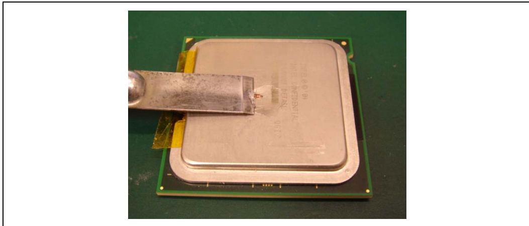
Figure 7-35. Removing Excess Adhesive from IHS
