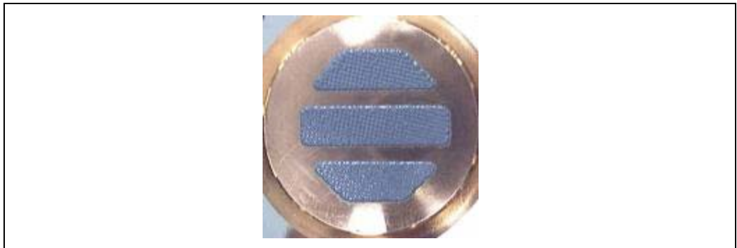
Figure 6-2. Bottom View of Copper Core Applied by TC-1996 Grease
