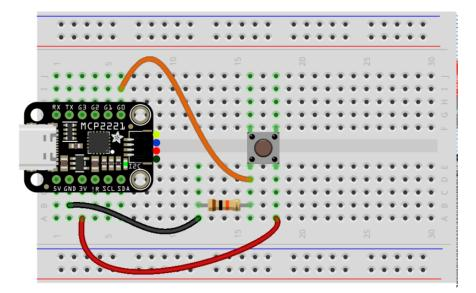
The GPIO pins do not have internal pull-up or pull-down support! If you need pull resistors, add them externally as shown here!
