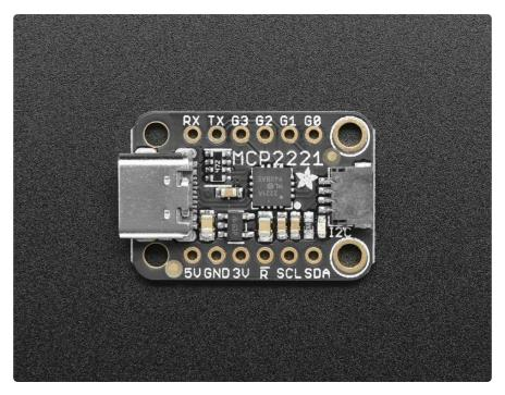
This guide will show you how to use an MCP2221(A) to connect to I2C sensors and breakouts from your desktop PC running Windows, Mac OSX, or Linux. The MCP2221 also allows for general purpose digital input and output (GPIO) for things like buttons and LEDs, analog to digital conversion (ADC), and digital to analog (DAC).
