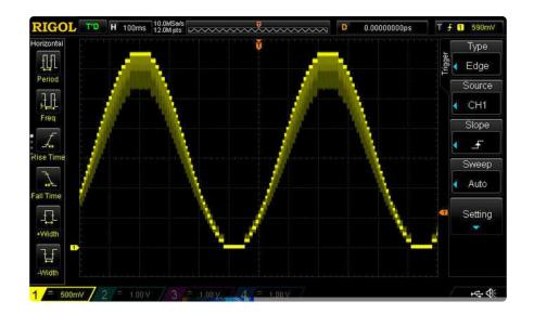
Note that even though the MCP221's DAC is only 5 bits, you set it using a 16 bit value to comply with the CircuitPython API.
