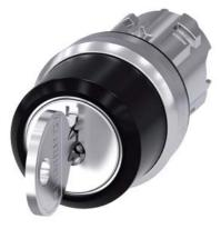
RONIS key-operated switch, 22 mm, round, metal, shiny, lock number SB30, with 2 keys, 3 switch positions I>O<II, momentary contact on the left, latching on the right, actuating angle 2x45°, 10:30h/12h/13:30h, key removal O, possible special locks: SB31, 421, 455, with laser labeling, upper case and lower case, always upper case at the beginning of the word
