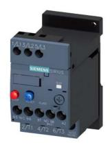
Overload relay 1.1...1.6 A Thermal For motor protection Size S00, Class 10 Stand-alone installation Main circuit: Screw Auxiliary circuit: Screw Manual-Automatic-Reset
