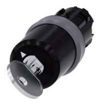
key-operated switch Siemens, 22 mm, round, plastic with metal front ring, lock no. LSG1, with 2 keys, 2 switch positions O<I, momentary contact type, actuating angle  $45^\circ$ , 10:30h/12h, key removal O, with laser labeling, upper case and lower case, always upper case at beginning of line
