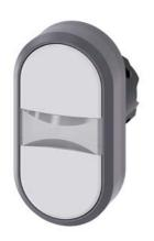
Illuminated twin pushbutton, 22 mm, round, plastic with metal front ring, white, white, Pushbuttons, flat, with laser labeling, upper case and lower case, always upper case at beginning of line
