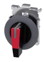
Selector switch, illuminable, 30 mm, round, Metal, matte, red, selector switch, long, front ring for flush installation, 3 switch positions I>O<II, momentary contact type, actuating angle 2x45°, 10:30h/12h/13:30h, with laser labeling, upper case and lower case, always upper case at beginning of line
