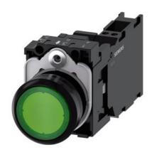
Illuminated pushbutton, 22 mm, round, plastic, green, pushbutton, flat, momentary contact type, with holder, 1 NO+1 NC, LED module with integrated LED 110 V AC, spring-type terminal, with laser labeling, inscription or symbol Customer-specific selection with SIRIUS ACT configurator (CIN)
