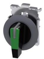
Selector switch, illuminable, 30 mm, round, Metal, matte, green, selector switch, long, front ring for flush installation, 3 switch positions I>O<II, momentary contact type, actuating angle 2x45°, 10:30h/12h/13:30h, with laser labeling, upper case
