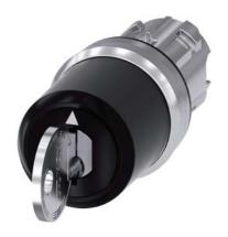
Key-operated switch IKON, 22 mm, round, metal, shiny, lock number 360012K1, with 2 keys, 3 switch positions I>O<II, momentary contact type, actuating angle 2x45°, 10:30h/12h/13:30h, key removal O, with laser labeling, upper case and lower case, always upper case at beginning of line
