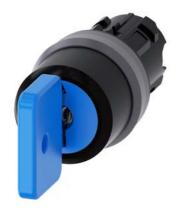
Key-operated switch O.M.R, 22 mm, round, plastic with metal front ring, lock number 73038, blue, with 2 keys, 3 switch positions I-O<II, left latching, right momentary contact type, actuating angle 2x45°, 10:30h/12h/13:30h, key removal O, with laser labeling, inscription or symbol Customer-specific selection with SIRIUS ACT configurator (CIN)
